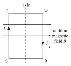
A coil, mounted on an axle, has its plane parallel to the flux lines of a uniform magnetic field B, as shown. When a current I is switched on, and before the coil is allowed to move,
