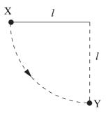
A ball of mass m, which is fixed to the end of a light string of length l, is released from rest at X. It swings in a circular path, passing through the lowest point Y at speed  $\upsilon$ . If the tension in the string at Y is T, which one of the following equations represents a correct application of Newton's laws of motion to the ball at Y?
