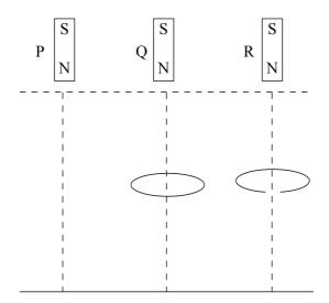
Three identical magnets P, Q and R are released simultaneously from rest and fall to the ground from the same height. P falls directly to the ground, Q falls through the centre of a thick conducting ring and R falls through a ring which is identical except for a gap cut into it. Which one of the statements below correctly describes the sequence in which the magnets reach the ground?
