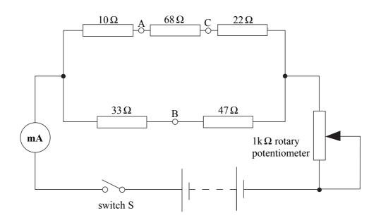
In each arm of the parallel sections of the circuit, a 4 mm round socket forms the common junction between a pair of resistors. These should be clearly labelled 'A', 'B' and 'C', as shown.
