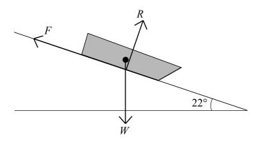
The three forces acting on the sledge are weight, W, friction, F, and the normal reaction force, R, of the ground on the sledge.
